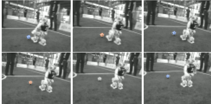
Fig. 5: A sequence of images captured while observing a kicked ball during a test game. Detected balls are denoted by circles of different colors, depending on the detector response: orange means a high probability that the detected object is actually a ball, blue means a medium probability. As one can see in this example sequence, rolling balls cannot be detected robustly. Please note that the images have been significantly compressed for logging purposes.
