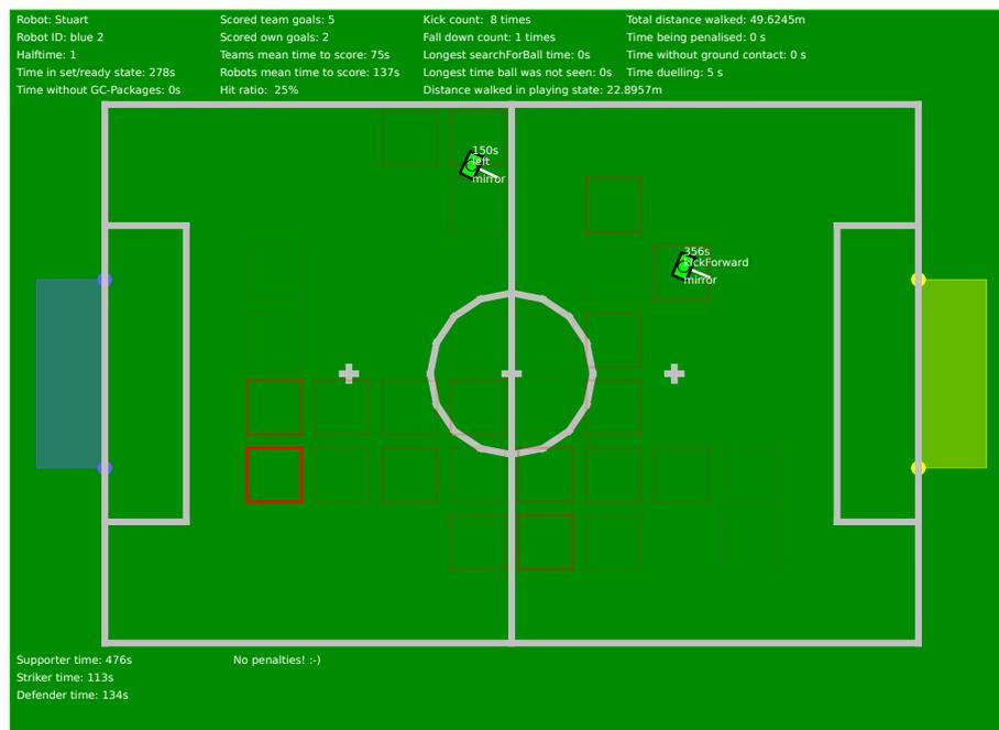
Figure 6.17: The red grid represents a robot's positional distribution. From the green robot poses, goals were scored.
