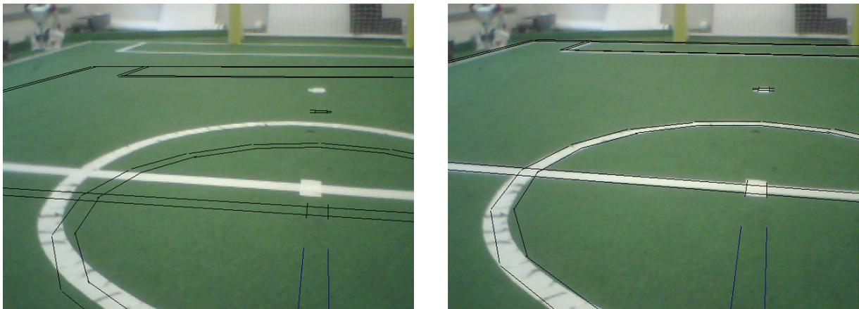
Figure 4.4: Projected lines before (left) and after (right) the calibration procedure
