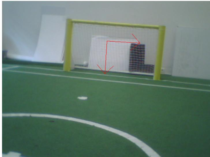
Figure 4.5: Origin of the *ImageCoordinateSystem*
