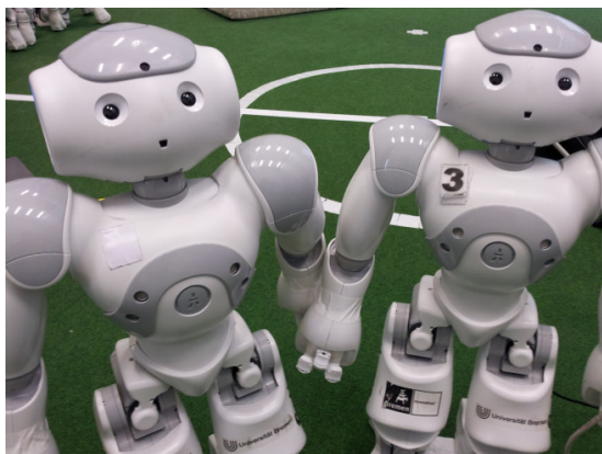
Figure 4.20: The left arm of the left robot is blocked and thus pushed back.
