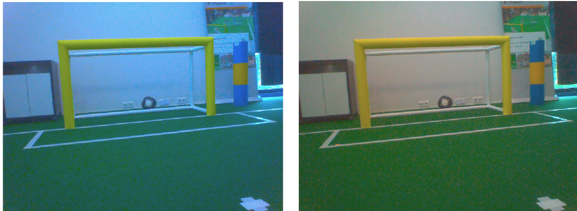
Figure 2.2: The left figure shows an image with improper white balance. The right figure shows the same image with better settings for white balance.
