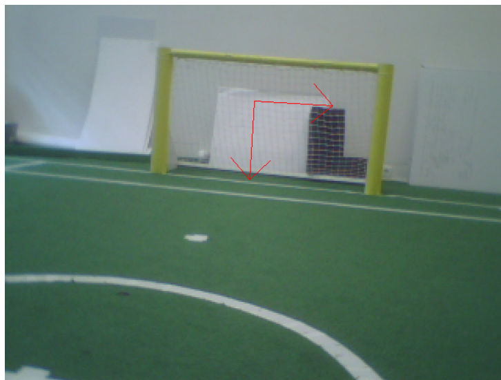
Figure 4.4: Origin of the ImageCoordinateSystem
