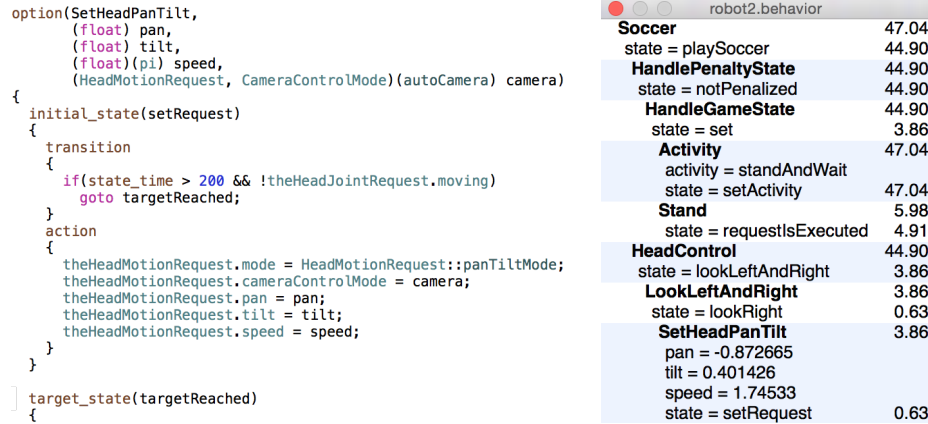
Fig. 6: The behavior view shows the actual parameters, e. g. of the option SetHeadPanTilt (left: source, right: view). The display of values equaling default parameters (specified in a second pair of parentheses) is suppressed. On the right of the view, the number of seconds an option or state is active is shown.
